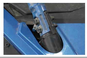
2. For multi passenger vehicles only, on the B-pillars you must inspect for the presence of 4 total bolts and nuts, and ensure the fasteners have been tightened by checking that the flanges on the bolts and nuts are contacting the mating surface on the ROPS and chassis.
