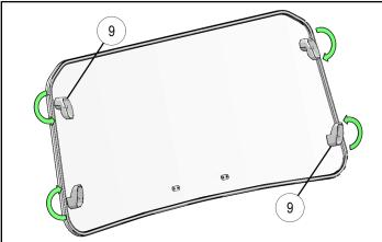
Install windshield 6 by inserting brackets 7 into newly cut slots (E) as shown. Pivot windshield into ROPS, then turn handles 9 to locked position (perpendicular to sides of windshield) as shown.
