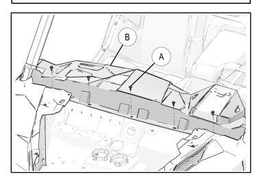
c. Slide upper dash panel (B) to rear, disengaging eight spring clips (C) retaining upper dash panel to main dash panel (D) as shown.
