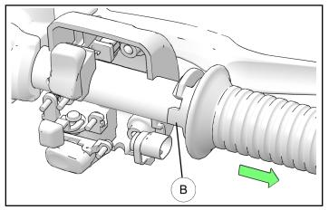
Install new RH throttle tube/grip (2) on handlebar. Ensure to line up slots in throttle tube (C) to throttle housing.
