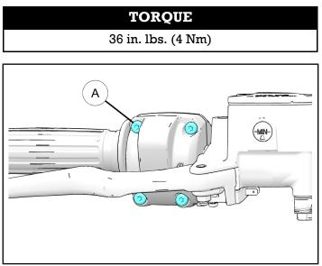
6. Remove two Torx<sup>®</sup> bolts (A) from LH switch cube and remove switch housing.
