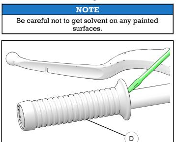
8. Firmly grasp LH grip (D) and remove from handlebar.
