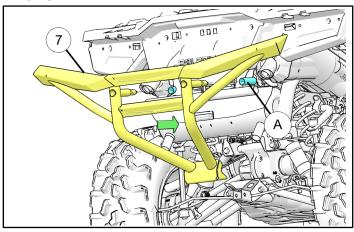
Slide the bumper mounting plate (a) with nuts facing down into the gap between the top of A-arm pivot and the frame (B). Insert screws (2) with lock washers (3) and flat washers (4) through the bumper (7) and vehicle frame (B) and thread into the bumper mounting plate (a). Tighten both screws (2) to below specification.
