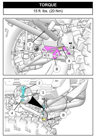
5. Tighten screws ① at this time to below specification. Final rear bumper ⑦ installation is shown below.
