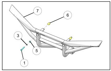
Install rear bumper assembly ⑦ by inserting wedge mounts into the bumper mount tubes (A). Push on bumper. Do not tighten screws ① at this time.
