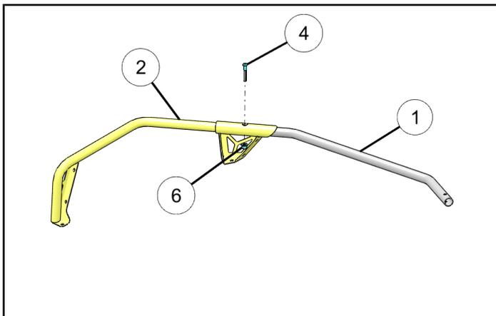
3. Repeat Step 2 for RH rack extender ③ installation.
