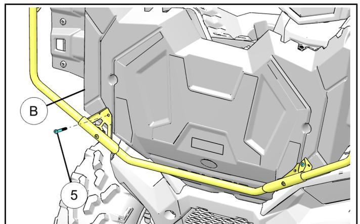
10. Close the front rack (B) along with rack extender assembly. Reinstall two screws (A) removed in Step 4 on front rack (B) through rack extender assembly as shown.
