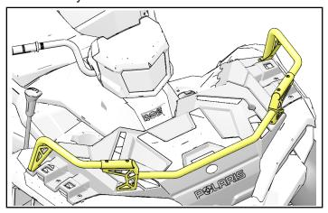
11. Reinstall two screws (B) removed in Step 4 on front rack (A) through the rack extender assembly as shown.
