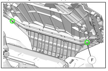
9. Place front rack extender assembly on front rack and install two screws ⑤ and nuts ⑥. Do not tighten fasteners.
