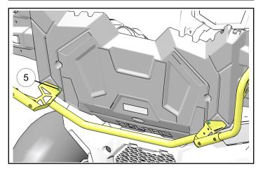
10. Close the front rack (A) along with rack extender assembly.
