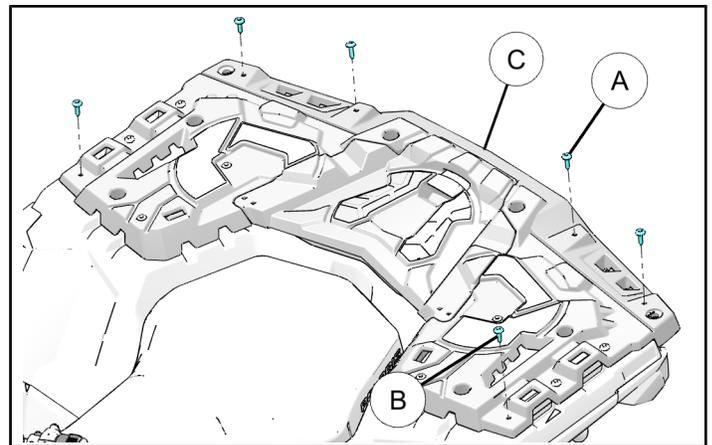
4. Install rear rack extender assembly on rear rack as shown and install four screws (A) removed in Step 3 to the rectangular rear rack extender ①. Tighten fasteners to specification.
