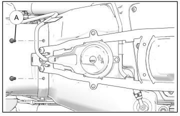
2. Place rear mounting tab ③ over mounting location, with loop facing down, and install with two retained seat mount fasteners (A).
