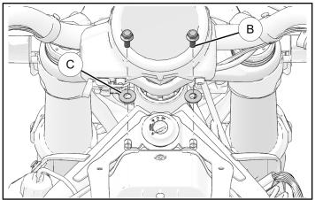
4. Place front mounting tabs ② over mounting location, with loops facing down, and install with two retained alignment bracket fasteners (B) and two retained washers (C).
