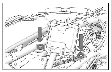
2. Place each tank cover on alignment bracket. Ensure each alignment tab is seated within corresponding tank cover hole.
