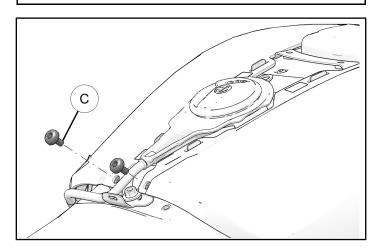
5. Place tab of center console into bottom bracket and flip down into installed position. Press firmly at adhesive pad locations to ensure each pad sticks to tank cover.
