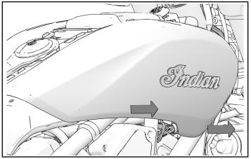
5. Pull each cover directly upward and free of alignment tabs.
