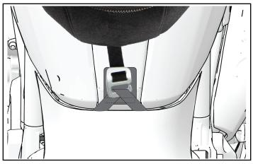
3. Lay mounting tabs against tank cover and hook front of tank bag.
