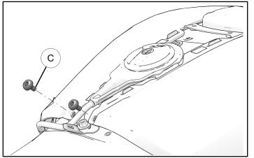
4. Pull bottom of each tank cover outward to disengage plastic rivets at two marked locations.
