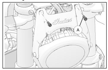
2. Remove and retain two screws (A) from bottom of headlight bracket.
