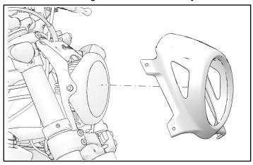
3. Remove and discard two fasteners © to remove lower head light cowl mounts from motorcycle.
