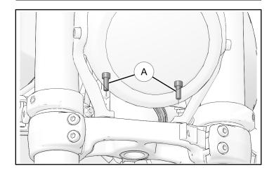
7. Reinstall top of headlight assembly with two retained headlight bracket fasteners (A).
