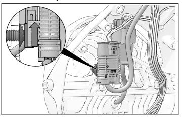
4. Disconnect headlight from chassis harness. Headlight connector will remain installed onto push-pin clip.
