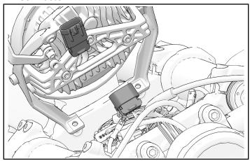
5. Re-mount electronic throttle control (ETC) connection onto push-pin clip.
