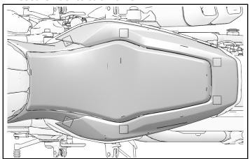
5. Remove seat and apply pressure to each pad for at least 10 seconds. Remove double-sided tape.
