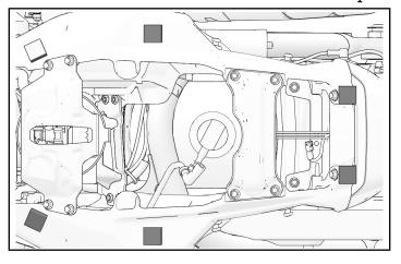
6. Reinstall seat and secure seat-rear to sub-frame with two retained seat fasteners (A).
