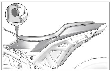
4. Apply pressure at six pad locations to ensure a secure fit onto sub-frame.
