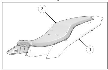
3. Flip seat and cowl upside down on clean surface. Loosely install seat to cowl with twelve seat fasteners (5) before torquing fasteners.
