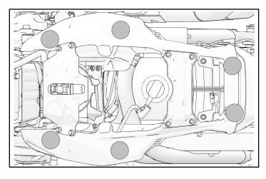
2. Place double-sided tape on six pads 3 and attach to ridges of seat cowl. Peel backing in preparation to apply to sub-frame. Ensure adhesive faces upward prior to installation.
