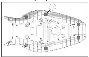
Slide front of seat cowl into position and engage with front seat bracket. Lower adhesive pads down onto sub-frame.
