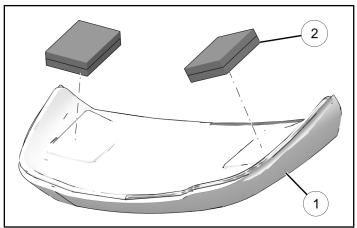
3. Peel backing from other side of hook-and-loop fasteners ②. Line seat pad ① with tracker seat and firmly press seat pad on tank cover to install. Remove seat pad and apply pressure to hook-and-loop fastener to completely adhere to tank cover.
