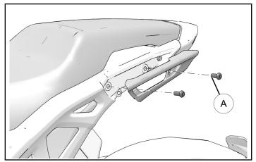
2. Remove and retain one seat fastener (B) from each side of motorcycle frame.
