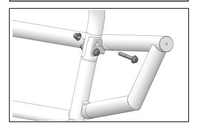
4. Pass two retained fasteners through brush guard bracket and intrusion bar. Install with two retained nuts.
