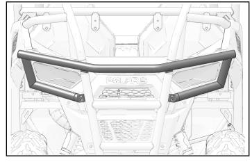
3. Pass two retained fasteners through brush guard bracket and intrusion bar. Install with two retained nuts.
