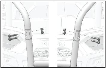
2. With an assistant, align rear brush guard with two intrusion bars.
