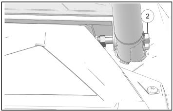
6. Loosely assemble clamps ② to brush guard with two bolts ④ and two nuts ③.
