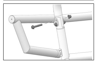
5. Loosely assemble clamps (2) to brush guard with two bolts (4) and two nuts (3).
