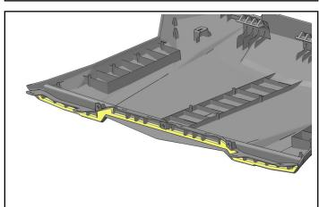
5. On rear roof panel ③ install three clip nuts ⑤ to standoffs at front of panel, and two clip nuts to standoffs at rear of panel.
