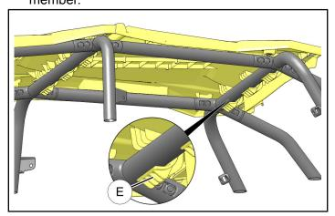
10. Secure left rear corner of rear roof panel ③ to ROPS using clamp ⑥ and screw ⑦. Repeat for right rear corner. Torque screws to specification.
