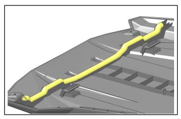
4. Peel adhesive backing from seam seal ②, then apply inside channel ③ at front edge of rear roof panel ③. Press firmly into place.
