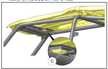
8. Slide entire roof assembly rearward until front hooks © lock into ROPS visor, then press rear edge of FRONT roof panel down until three middle hooks ® lock over B-pillar cross-member.
