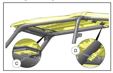
9. Press rear edge of REAR roof panel down until three rear hooks (E) lock over C-pillar crossmember.
