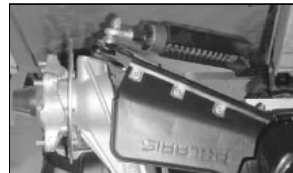
Figure 7 - Front anti-rotation installation (step 6.6)
