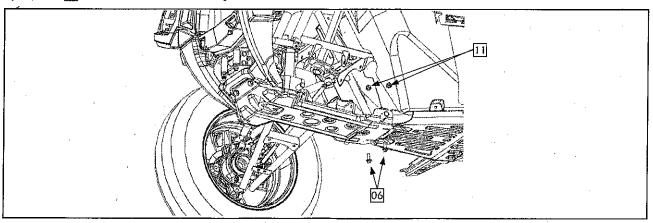
6. Finger tighten the front bolts completely. Torque all bolts and nuts starting by the rear bolts and finishing with the front bolts to avoid twisting the plate.
