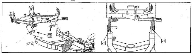
3. Place the tension spring 26 in the hook up 17. Insert the adjustment wire 16 in the open end of the spring then insert the eyebolt in the eyelet of the pushframe and fasten using one (1) M8-1.25 nylon nut 11 and one (1) M8 washer 01. IMPORTANT: Fully tighten the eyebolt using a screwdriver to retain the eyebolt from rotating in order to avoid twisting the steel cable.
