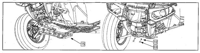
5. Fasten the rear part of the mount plate using two (2) M8-1.25 x 25 mm hex. flange bolts 06 with two (2) M8 flange nylon nuts 11. Screw the first threads only at this time.
