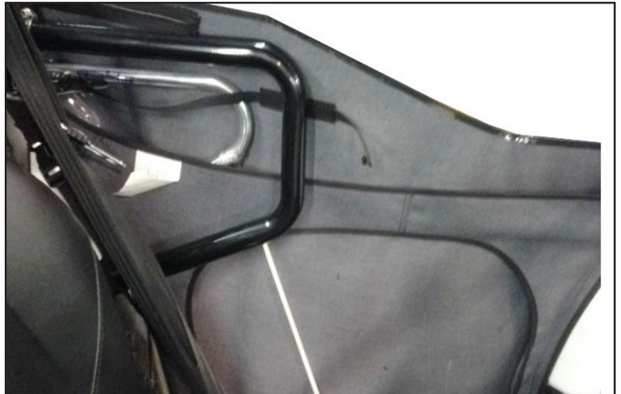
17. Tightly close the RHS door and adjust. Insert the ½" webbing strap (20) with the red webbing handle through the channel on the doors from front to back. Screw the ½" webbing strap to the latch using the supplied screw, threading it into the supplied knob (18).
