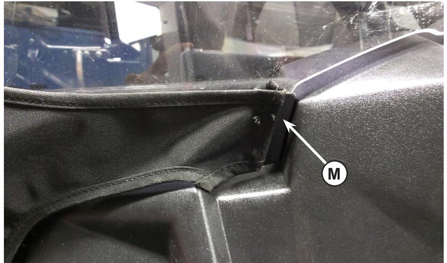
14. Attach the loop fastener at the upper and rear edges of each door fabric to the hook fastener on the frame. This will tighten the fabric on the frames. This attachment can be adjusted once the installation is completed to adjust the seal of the doors.
