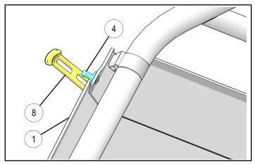
5. Torque all clamps screws ① to specification.
