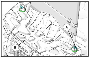
8. Using tangency of the washer (10), push washer into the corner of the box highlighted below. Use hole of the washer as a template to mark out the hole for drilling. Using 1/4" or 7mm drill bit, drill hole on front box cover (B) for spacer (9) installation.
