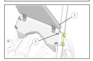
Move windshield ① into up position. Slide visor so that rubber strap bumpers ⑧ sit properly on the visor surface. Attach rubber straps to the ball studs ④. Snap the visor clamps into position.
