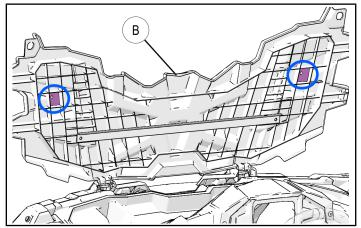
Install spacer (9) onto front box cover using screw
