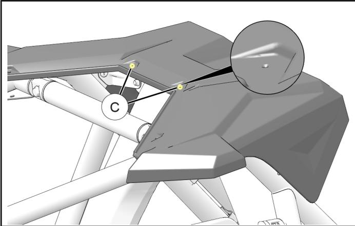
6. Loosely install FRONT of roof panel ① using two each 25 mm screws ⑦, steel washers ③, rubber washers ②, and nuts ⑥.
