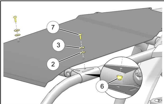
7. Loosely install MIDDLE of roof panel ① using two each 45 mm screws ④, steel washers ③, and rubber washers ② into clip nuts ⑤ or ⑩.
