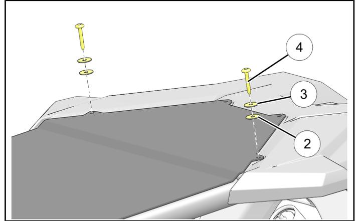
8. Loosely install REAR of roof panel ① using two each 45 mm screws ④, steel washers ③, rubber washers ②, and nuts ⑥.
