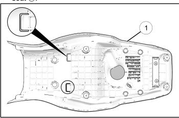
2. Tabs, identified in step 1 of this section, will slide beneath seat support bracket.
