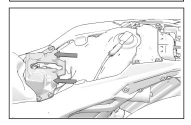
3. Slide aviator seat into seat support bracket and into front mounting bracket.
