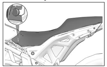
4. Secure rear of aviator seat with two retained screws (B).
