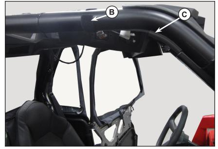
14. Roll up all windows, and close all zippers. Adjust all hook and loop fasteners on the fabric doors and door frames to tighten the fabric on the frames. The fabric can be relaxed or pulled tighter to adjust the positions of the seals around the door. When finished, the doors should have a tight seal with the vehicle.
