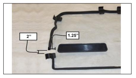
4. Install the ROPS attachment bracket to the C-Pillar, using a hose clamp, as show. The hinge of the bracket should face the outside of the vehicle. The hose clamp should seat directly beneath the horizontal ROPS bar. This should be finger-tight only; they will be adjusted during a later step.
