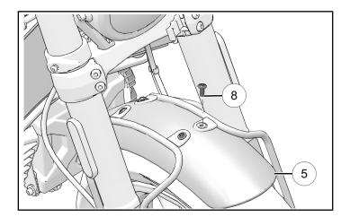
5. Torque mudguard mount hardware, loosely installed in steps 2 and 3 of this section.
