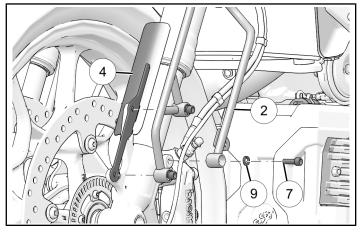
3. Loosely install RH mudguard mount ① and RH fork guard ③ with three washers ⑨ and three screws ⑦.
