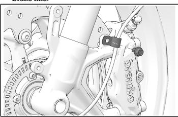
2. Loosely install LH mudguard mount ② and LH fork guard ④ with three washers ⑨ and three screws ⑦.
