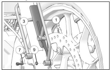
4. Place mudguard ⑤ beneath mudguard mounts and loosely install with four mud guard fasteners⑧ prior to torquing.
