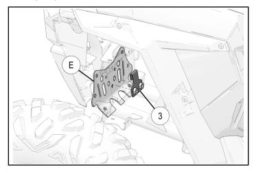
9. Position bumper ①, then loosely install screws ⑤ through washers ⑦, bumper, and chassis, into backing plate ③ as shown.
