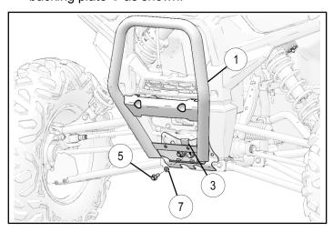
10. Loosely install screws ④ through washers ⑦, bumper ① and chassis, into nuts ⑥ as shown.
