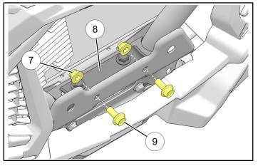
c. Torque all four screws to specification.
