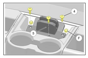
16. Clean installation surface for LH seal ② as required. Peel off adhesive backing, center seal over existing push pin rivet, then press firmly into place.
