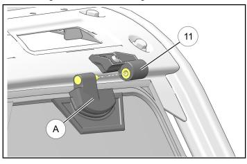
5. Assemble RH vehicle-side hinge ① to windshield-side hinge ⑧ by sliding pin into bushing.
