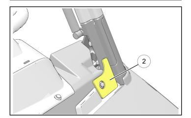
17. Close windshield and lock handle into base ⑤. Ensure windshield seal is adequately compressed and windshield opens/closes properly. Adjust as required.
