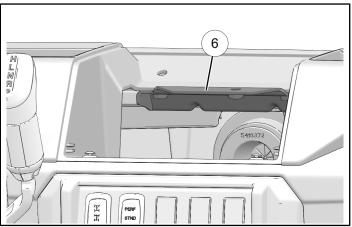
13. Position handle base ⑤ in upper dash cupholder so base nests into cupholder where angled surfaces meet at ⑪. Center handle base left to right in cupholder, then mark three holes ① in centers of slots.
