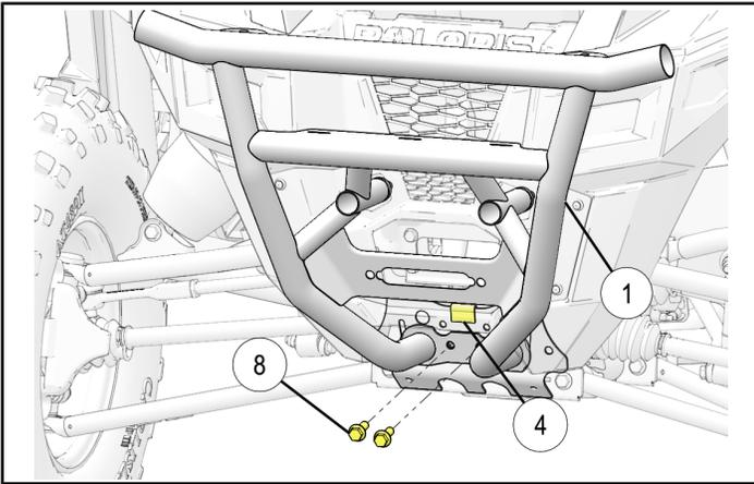
6. Torque all fasteners ⑦ ⑧ to specification.
