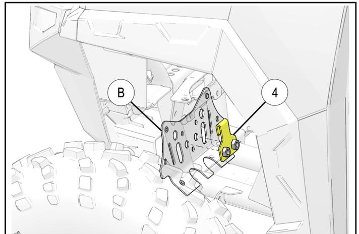
4. Loosely install upper portion of bumper ① to vehicle chassis using two bolts ⑦ and nuts ⑨ as shown.
