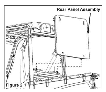
4. Clamp the mounts (PN 5439918) of rear panel on the Cab Frame Plate. Figure 3.
