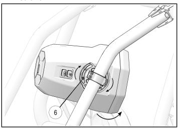
6. Connect long electrical harness from master audio pod ② to harness from slave audio pod ①. Secure harnesses to C-pillars and C-pillar cross member as required to prevent contact with sharp edges.
