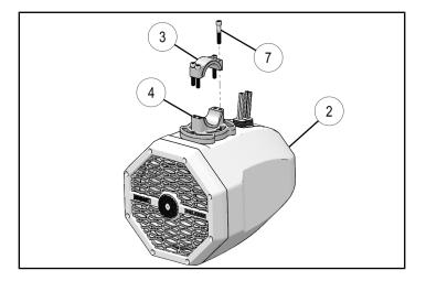
Insert bushing ® into upper clamp ③ and lower clamp ④, then install master audio pod ② to RH ROPS C-pillar by loosely assembling upper clamp ③ to lower clamp ④ using retained screws ⑦.
