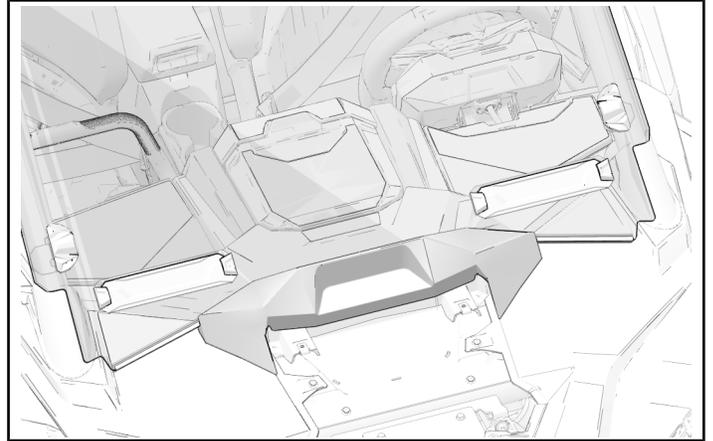
3. With windshield in correct position, secure to ROPS with four Lock & Ride® clamps.
