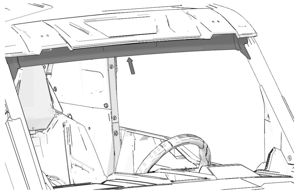
2. Remove backing paper and install windshield seal 7 on visor plate. Bottom edge of seal should be flush with bottom edge of visor plate.
