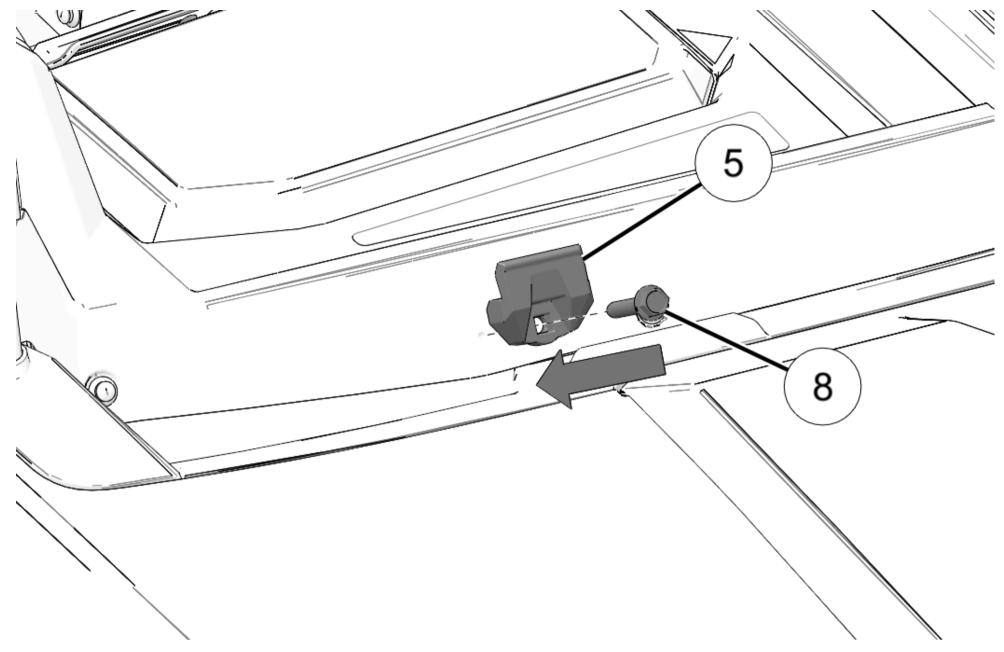
5. Set windshield 1 on the lower clamps and into position in the opening.
