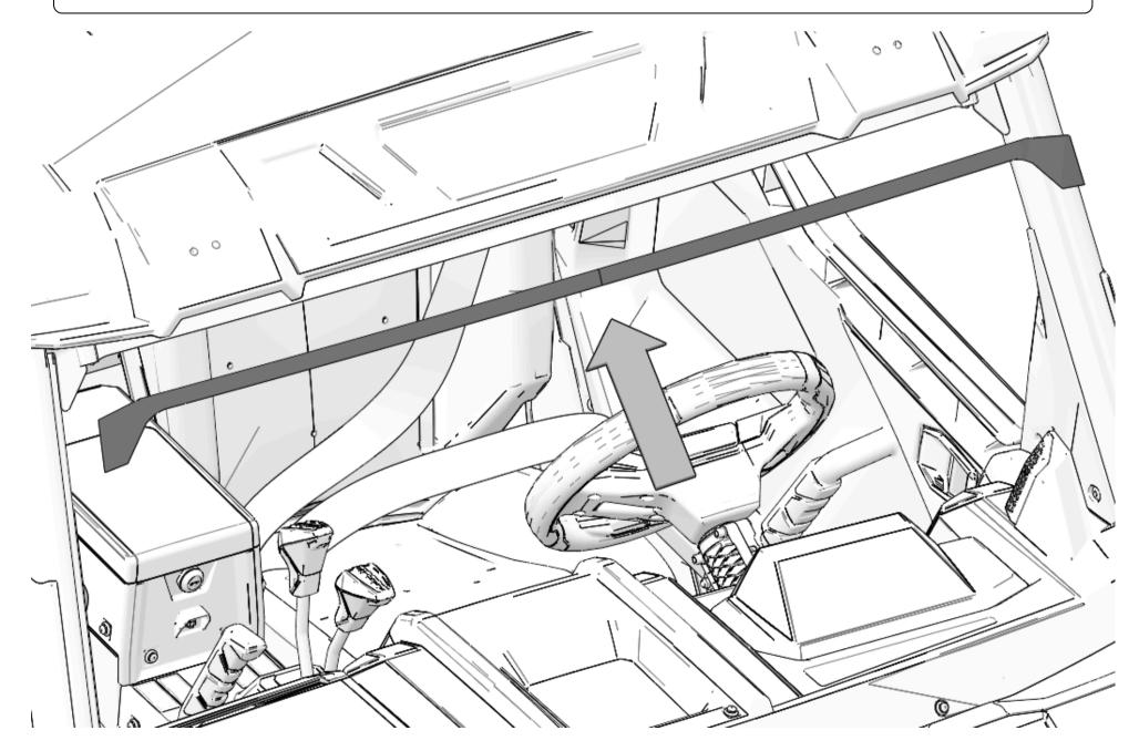
3. Locate two dimples on dash at bottom of windshield opening. Drill hole through each dimple.
