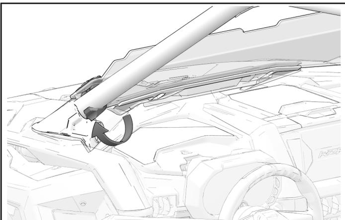
4. Windshield may need repositioning. If needed, release clamps and move windshield upwards along roll-cage.
