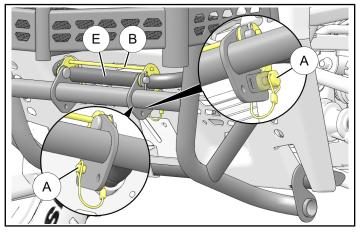
5. Secure upper hook assembly (B) to upper hook brackets using two wire lock pins (A).
