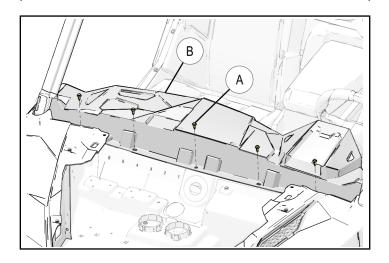
c. Slide upper dash panel (B) to rear, disengaging eight spring clips (C) retaining upper dash panel to main dash panel (D) as shown.
