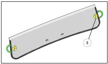
Install windshield (5) by inserting brackets (6) into newly cut slots (E) as shown. Pivot windshield into ROPS, then turn handles (8) to locked position (perpendicular to sides of windshield) as shown.
