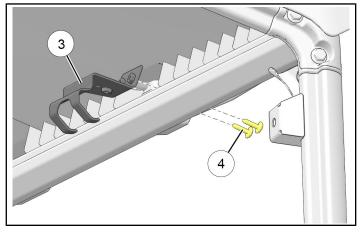
12. Secure front roof panel to ROPS visor using two screws 10.
