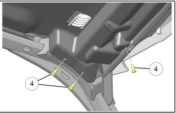
d. If installing optional front light, then refer to instructions included with light. Otherwise, loosely install two each screws (1) and washers
