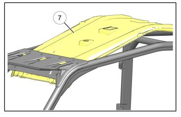
5. Align all six liner holes (E) and (F) with nut clips in ROPS structure, mark four upper holes (D), then remove liner. Drill 5/16 inch (8 mm) holes through liner at marked locations, then reinstall liner.
