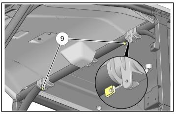
b. Insert rear edge of rear roof liner (6) above Cpillar cross-member, then slowly tip liner up, inserting LH and RH liner edges between ROPS and roof seal.
