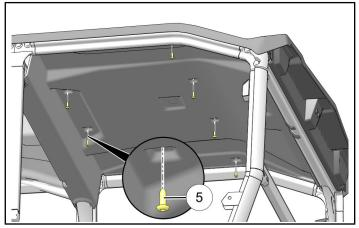
e. Loosely install two screws ④ rearward through roof liner into previously installed clip nuts ⑨.
