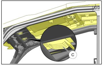
9. Slide entire roof assembly rearward until three hooks C lock into ROPS visor, AND three hooks
