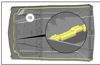
8. Using two people lift entire roof assembly as a single unit, supporting front and rear panels to prevent bending, then lay on top of ROPS.
