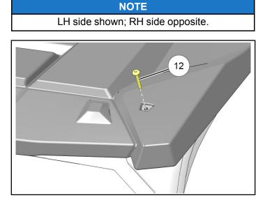
13. Torque screws ④ and ⑫ to specification.
