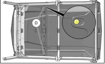
3. Clean underside of front and rear roof panels as required to ensure proper foam tape adhesion.
