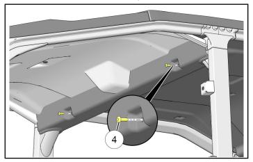
f. Tighten all screws ④ and ⑤. Do not overtighten screws.
