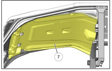
c. Loosely secure front of roof liner to ROPS bracket and roof using three screws ④. Repeat for RH side.
