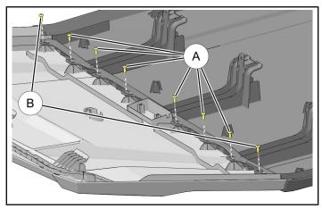
6. Torque screws  $\bigcirc$  to specification.
