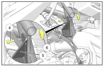
4. Lift bumper ① into position, then loosely install upper end of bumper to upper LH mount bracket
