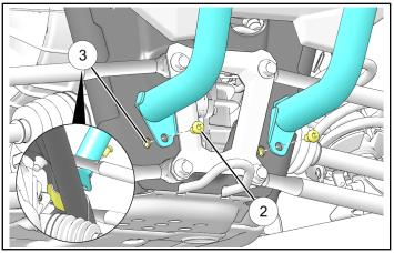
6. Torque screws to specification.
