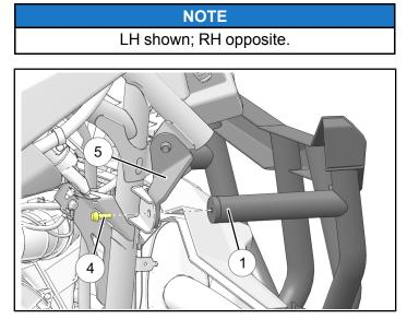
Hold attach plate ③ in position on forward side of transmission/suspension mount plate, then loosely install bumper to plates using screw ④. Repeat for RH side.
