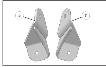
Loosely install upper LH mount bracket (5) to vehicle chassis using screw (4) and spacer (with weld nut) (6). Repeat for RH side using upper RH mount bracket (7).
