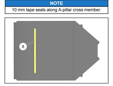
c. Peel adhesive backing from 5 mm thick foam tape (9) and apply to SIDES and REAR of roof panel on INSIDE edge of alignment marks, butting up to foam tape (8) on each end.
