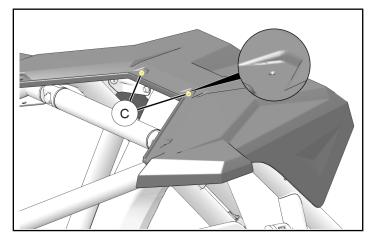
6. Loosely install FRONT of roof panel ① using two each 25 mm screws ⑦, steel washers ③, rubber washers ②, and nuts ⑥.
