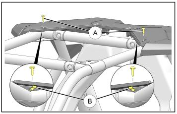
5. Drill two 5/16 inch (8 mm) holes through high intake cover at marked locations ©.
