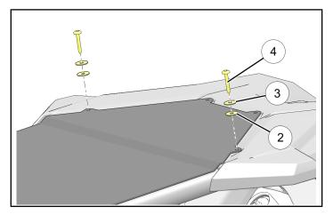
Loosely install REAR of roof panel ① using two each 45 mm screws ④, steel washers ③, rubber washers ②, and nuts ⑥.
