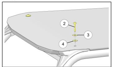
7. Loosely install rear of roof ① using two each 25 mm screws ⑥, steel washers ③, and rubber washers ④ as shown. Ensure steel washer is beneath screw head, and rubber washer is against roof.
