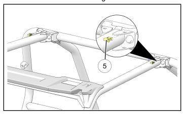
OPTIONAL: Two existing clip nuts (B) on outer flanges of front frame may remain if in good condition. Otherwise, replace with new clip nuts (5).
