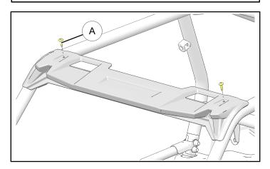
3. Install two clip nuts ③ to outer flanges of rear frame as shown. Inner flanges will not be used.
