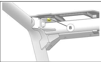
4. Install one clip nut ④ to each of six clamps ③ as shown. Ensure proper orientation: Threaded portion of clip nut is on lower surface of clamp.
