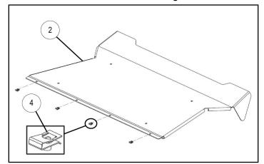
b. If not already accomplished by factory: Install 3 mm foam tape ③ across front edge from LH to RH sides. Notch or punch holes through tape at four clips nuts ④ to facilitate fastener installation.
