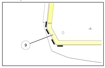
d. Apply 10 mm foam tape (10) to six remaining locations (LH/RH sides of front and rear panels, B-pillar cross member, and C-pillar cross member). Tape should be applied on INSIDE edge of alignment marks as shown. Trim as required.
