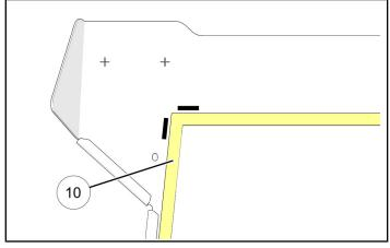
9. Lift entire roof assembly as a single unit, supporting front and rear panels to prevent bending, and lay on top of ROPS.
