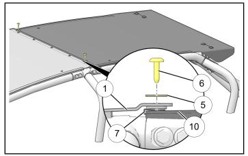
Install clip nut to each clamp as shown. Ensure proper orientation: threaded portion of clip nut must extend in same direction as curved portion of clamp.
