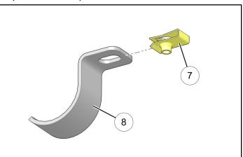
9. Loosely install three clamps (8) (with clip nuts) to roof panel seam at B-pillar using screw (6) and washer (5) at each clamp.
