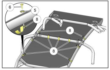
10. Ensure roof panels are centered on ROPS, then torque all roof screws (6) to specification.
