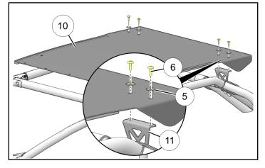
Lay FRONT roof panel ① on top of ROPS, then loosely install LH plate ④ (with RZR<sup>®</sup> stamping) and left front corner of roof to ROPS A-pillar crossmember using two each screws ⑥ and washers ⑤.
