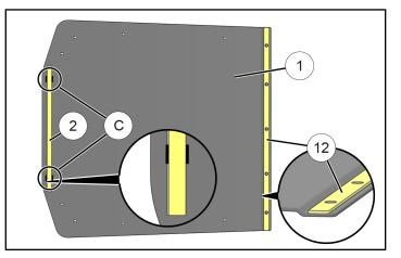
d. Lay 21.0 inch (533 mm) foam tape ② along front of panel, centering tape between BOTH pairs of alignment marks ⓒ (left to right, and front to rear).
