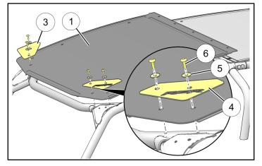
Loosely install rear edge of FRONT roof panel 1 to front edge of REAR roof panel 1 using two each screws 6 and washers 5 into previously installed clip nuts 7.
