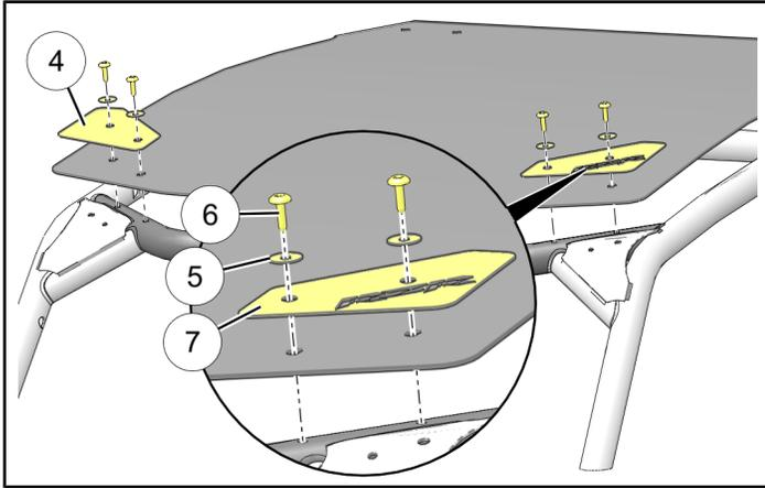
6. Loosely install rear of roof to brackets ⑧ using four each screws ⑥ and washers ⑤.
