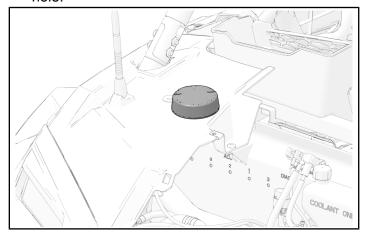
3. Secure V2V antenna with slip-nut.
