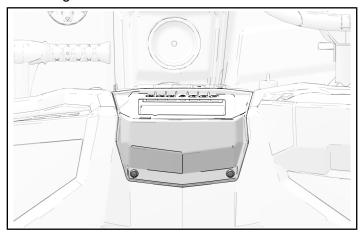
2. Remove four fasteners from top dashboard panel. Remove panel from vehicle.
