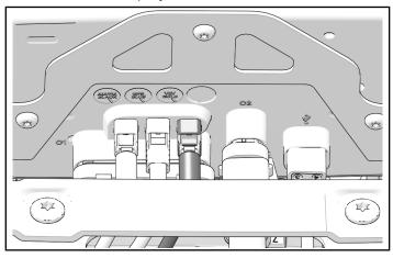
4. Secure antenna harness to chassis harness with cable ties ③.
