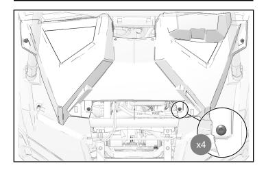
2. Install top display/storage bezel to top dashboard panel with two push-pin rivets.
