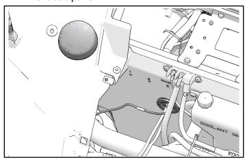
Route antenna harness to Ride Command<sup>®</sup> display. Connect antenna harness to back of Ride Command<sup>®</sup> display.
