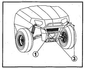
4. Attach the lower mounts of the Brushguard to the vehicle frame using two 6mm x 90mm flange head bolts (4).
