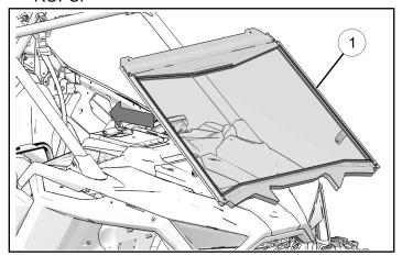
2. Install top of windshield ① to ROPS brackets with two fasteners ③ and two nuts ⑤.
