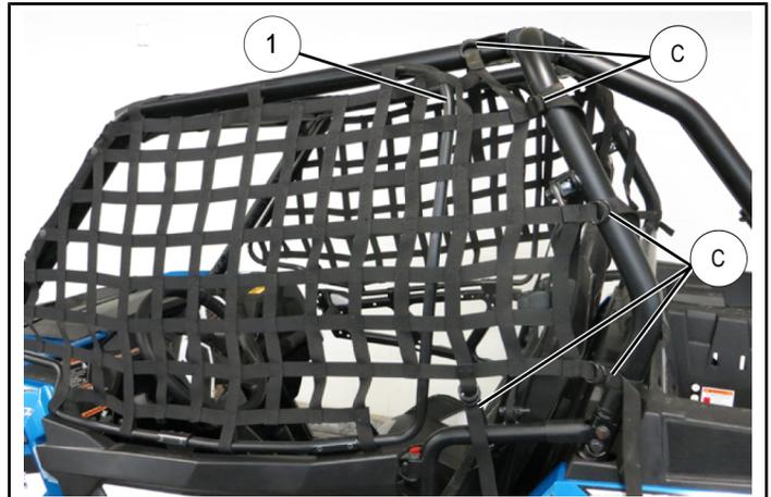
6. Open door to ensure straps do not restrict door operation. Adjust straps as required.
