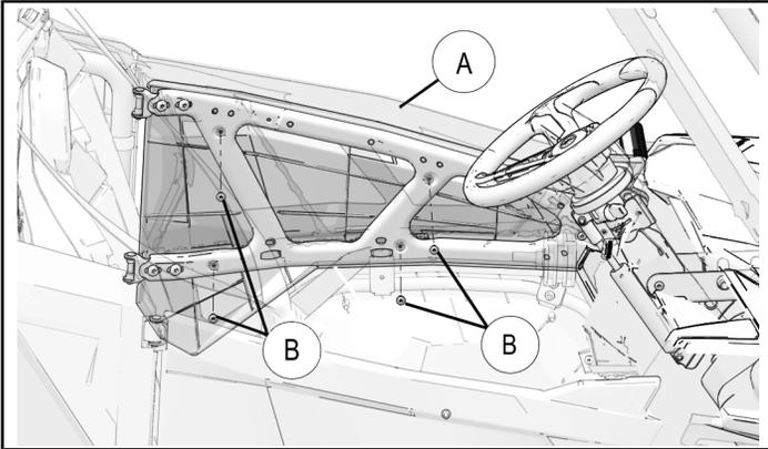
3. Loosely install upper door frame (1) to each door using bolts (3), washers (5), and nuts (4) as shown.
