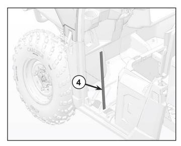
16. Install brake cylinder foam (11) on to the front floor body as shown. Ensure the proper placement of seal.
