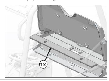
4. For Kit PN 2880508: Install rear lower close off foam (2) at the proper position on to the close off panel ensuring the clean surface as shown in figure.
