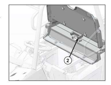
5. For Kit PN 2880508: Install two B pillar foams (13) LH and RH by pressing firmly against the metal surface. LH side shown in figure.
