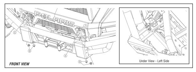
2. Position and fasten the middle section of the front brushguard ① onto the left ④ and right ⑤ supports installed in **step 1** using (4) M8-1.25 X 20 mm flange bolts ⑦ and (4) M8-1.25 flange nylock nuts ⑨ (finger tighten at this time).
