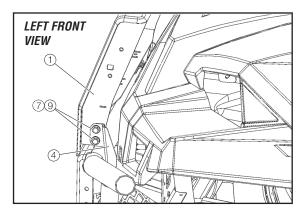
3. Position the taper block (a) onto the end of the left brushguard section (a) and fasten using a M8-1.25 X 130 mm Allen socket machine screw (a) and a M8 lock washer (b). Tighten until the taper block (b) leaned against the left section.
