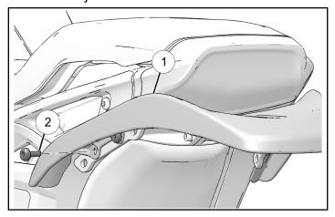
2. Complete installation with four nuts ③. Counterhold nuts ③ while torquing screws ②.
