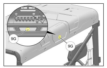
b. From outside cab use 1.25 in (32 mm) hole saw, centered on pilot hole, to drill forward through roof panel.
