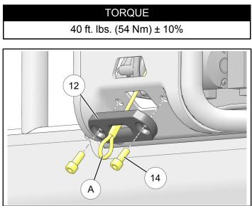
6. Install hook (13) to loop (A) using clevis pin, then secure with cotter pin.
