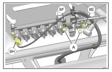
2. Torque two nuts (A) to specification, then reinstall red boot over post **BAT +**.
