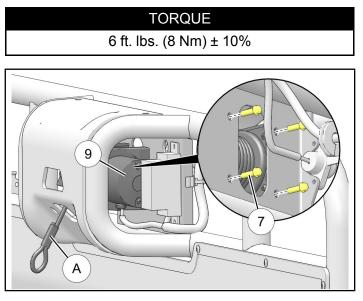
2. Install contactor 9A to frame using two each screws (1) and nuts (8). Tighten screws.
