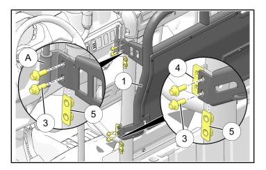
Loosely install LOWER LH corner of frame ① to ROPS using two screws ③, spacer ④, and nut plate ⑤.
