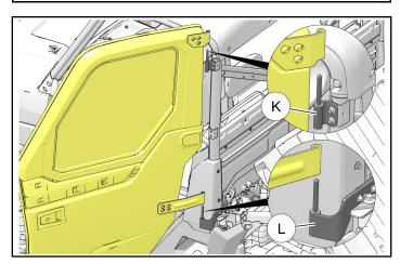
c. Remove UPPER chassis-side hinge (k) by removing two screws (m) and nut plate (n). Retain hinge (with nylon washer). Screws, nut plate, and conical spring washers (if installed) will not be reused.
