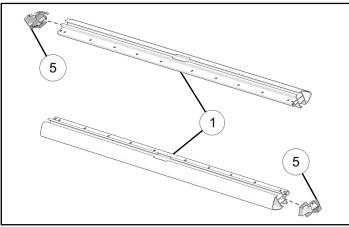
3. Insert right-hand corner base pieces ⑤ inside the channel on each end of extrusion ①.
