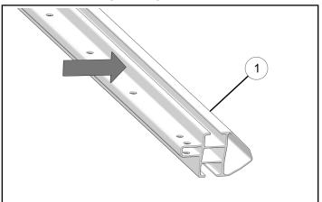
2. Install two right-hand corner base pieces ⑤ to front and rear extrusions ①.
