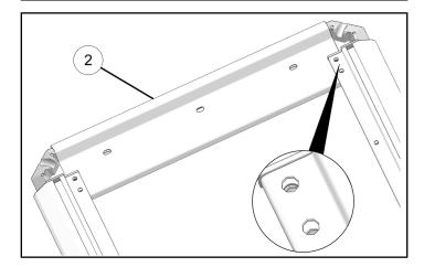
7. Loosely install side extrusions with eight bolts 10.
