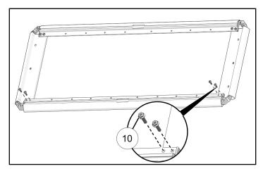
8. Loosely install four platform planks 3 to platform frame assembly with sixteen bolts 10.
