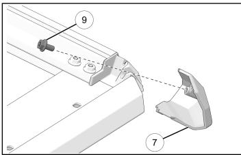
10. Torque all bolts with torque tool ①.
