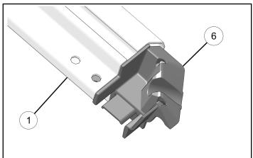
6. Slide two side extrusions ② into each corner base.
