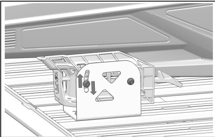
3. Counter hold nuts and torque two screws ⑤ to specification.
