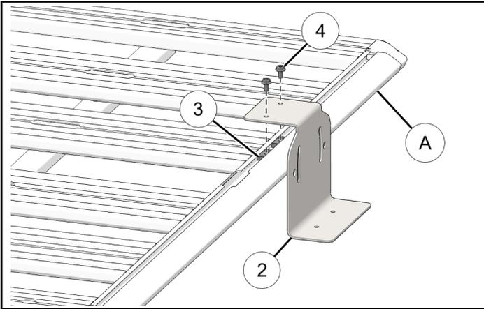
4. Attach pioneer u-bracket ① to pioneer side bracket ② with two screws ④.
