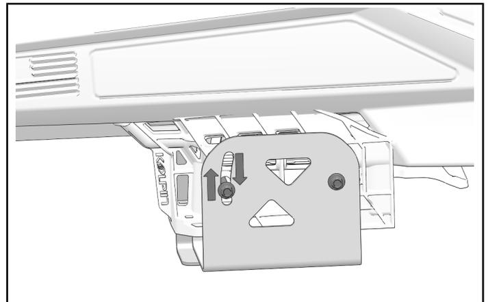
5. Counter hold nuts and torque two screws ⑤ to specification.
