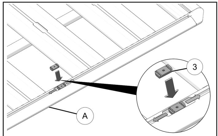
2. Slide both channel nuts ③ to desired location.
