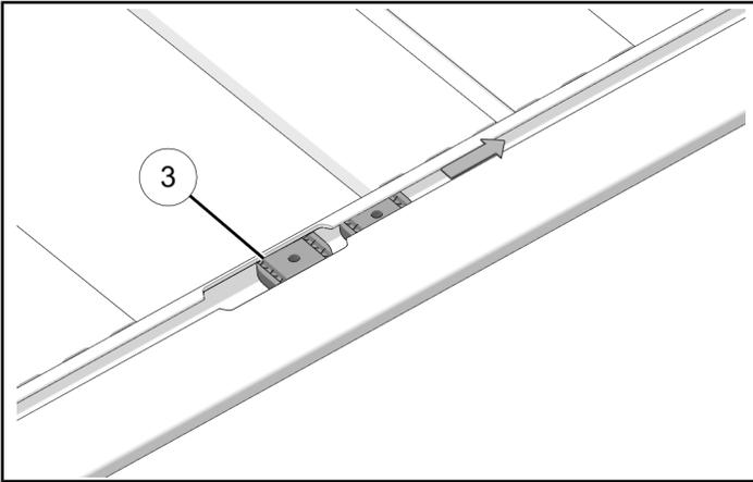
3. Loosely install pioneer side bracket ② to platform rack frame ① with two screws ④ and the two channel nuts ③.
