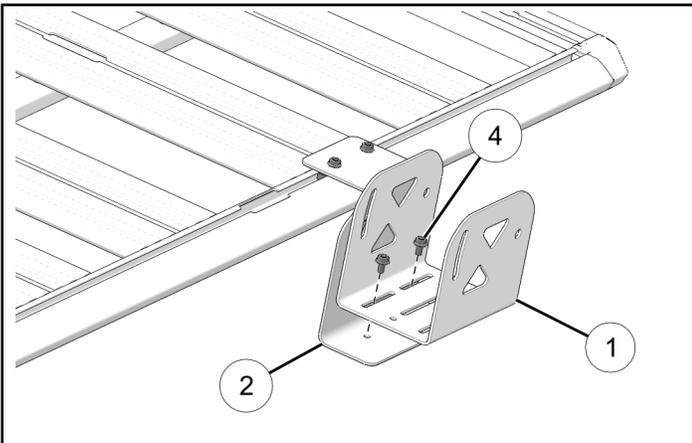
5. Torque two pioneer side bracket screws ④ with torque tool ⑤ or torque to specification using socket set.
