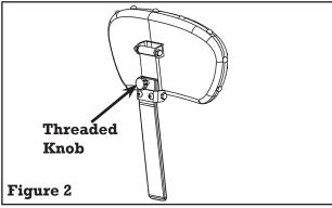
WARNING: Post must be engaged in a detent. Do not set height higher than the tallest detent. Periodically check all fasteners to ensure they are remaining tight.
