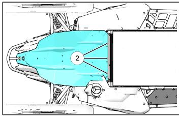
8. Install the two larger self drilling screws ③ into the middle of the skid plate as shown.
