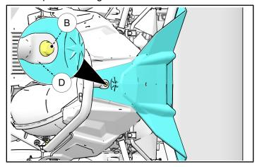
7. Install the three smaller self drilling screws ② in the rear of the skid plate as shown.
