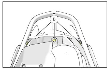
4. Loosen the two rear bumper mounting fasteners © but do not remove.
