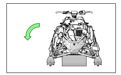
6. Position the High Coverage Skid Plate under the front bumper mounting tab ① as shown and insert the original center bumper mounting bolt ® and loosely install the nut you previously removed onto bumper mounting bolt.
